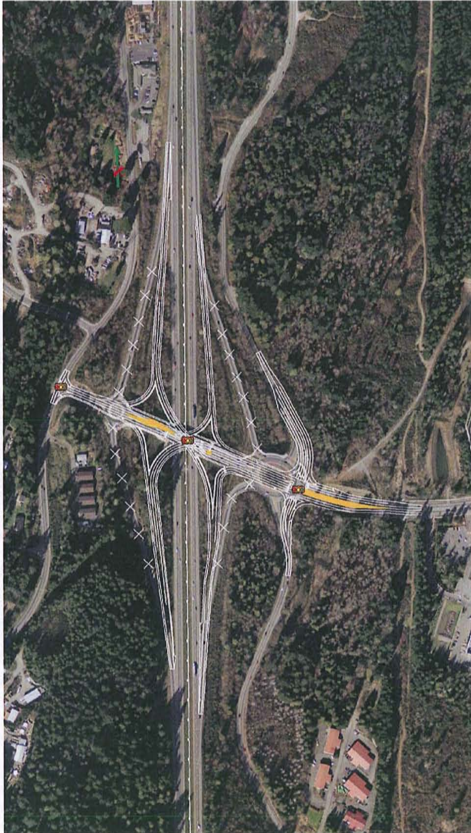
EXHIBIT 8: SINGLE POINT URBAN INTERCHANGE (SPUI)
