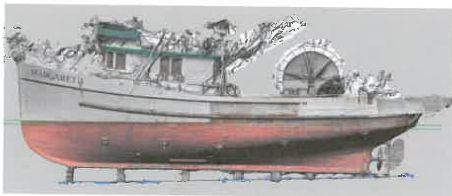
A composite computer model of the Margaret J comprised of over 650 digital photographs. The first step, in what's termed photogrammetry, is capturing the lines and table of offsets for a vessel.
